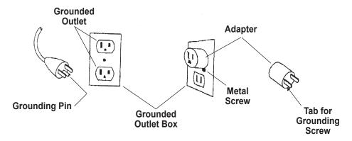
Extension Use only a 3-wire extension cord that has a 3-blade grounding plug, and a 3-slot receptacle that accepts the plug on the product. Verify the extension cord is not damaged. When using an extension cord, use one that is heavy enough to carry the current the product draws. For lengths less than 25 ft., use 18 AWG extension cords. An undersized cord results in a drop in line voltage, loss of power, and overheating.
