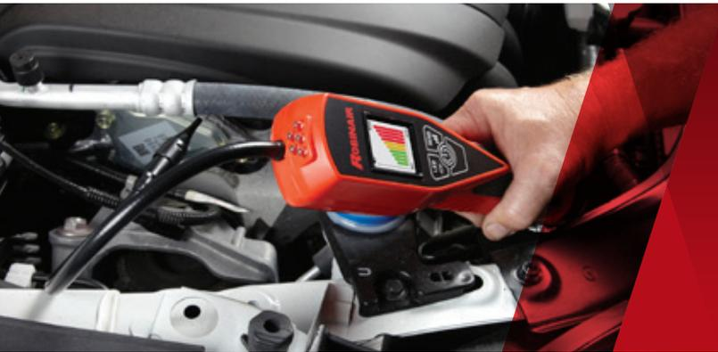
Leaking refrigerant, especially 1234yf, can be an expensive problem. Using a 5% hydrogen/ 95% nitrogen tracer gas mix can help find leaks faster for repair and recharge of the A/C system, without losing refrigerant.
